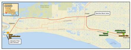
This diagram depicts the TransCameron natural gas pipeline and its general vicinty along the pipeline route. Pipeline markers are used to locate the general location of a pipeline but always call 811 to have all utilities marked before digging.
